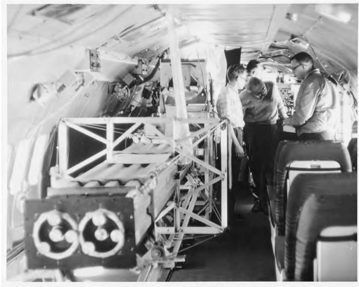
Solar spectrometer (left side) on the NASA CV-990 aircraft for infrared spectroscopy. A. B. Thompson, G. P. Kuiper, G. T. Sill D. Cruikshank photo (July-August, 1968) See LPL Communication No. 126, 1968
