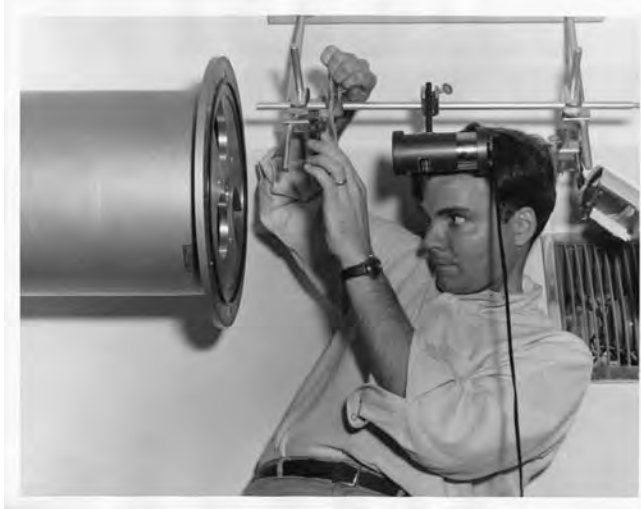
Photos 15 and 16. Photo 15 shows graduate student Toby Owen with the small (62-ft) absorption cell in the original Lunar and Planetary Lab facility. He used data obtained with that tube for his dissertation on planetary spectroscopy (LPL Photo). Photo 16 shows the larger 40-m absorption cell under construction in the new Lunar and Planetary Laboratory (now the Kuiper Building). Photo by D. Cruikshank
