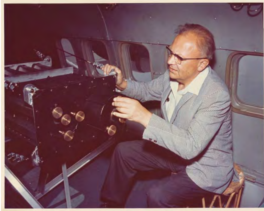
Photo 20. G. P. Kuiper aboard the NASA Convair 990 (Galileo) with the large solar spectrometer used for the creation of a high-resolution atlas of the Sun with minimal atmospheric interference. NASA Ames Research Center photograph.
